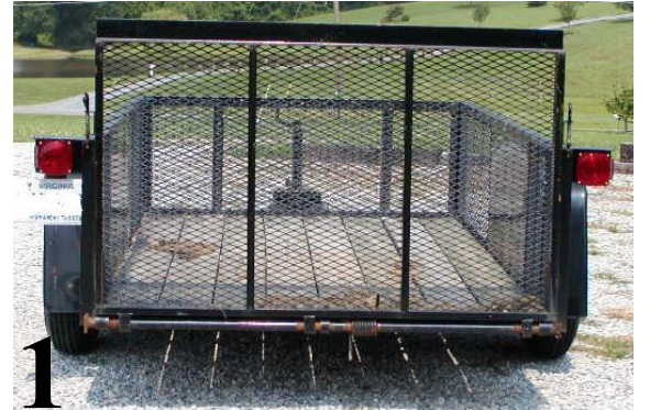
PHOTO 1: VIOLATION - This trailer has no reflectors or reflectorized tape.
