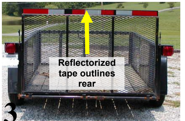
PHOTO 3: NO VIOLATION - This trailer has 100+ inches of reflectorized tape.
